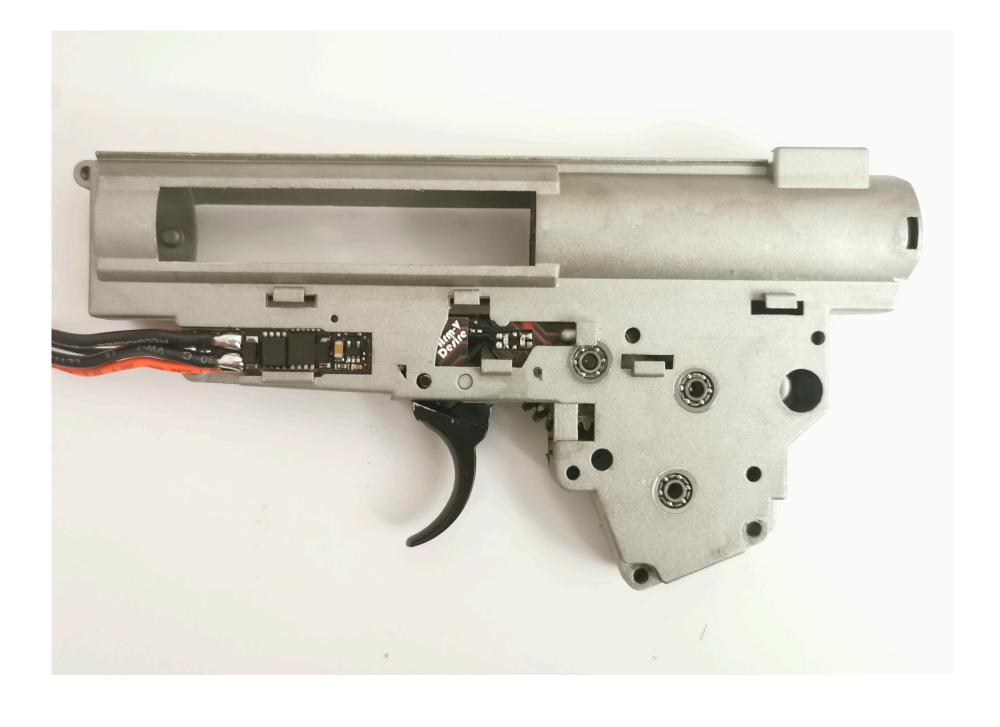
INSTALLATION OF DESIRE V3 INTO GEARBOX
