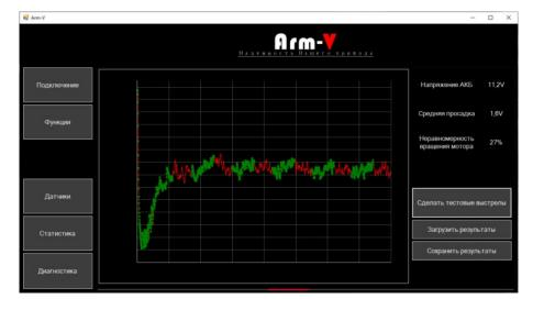
The color on the graph indicates the status of the gear sensor. A completely green graph means the gear position sensor is not working. This can be if:
