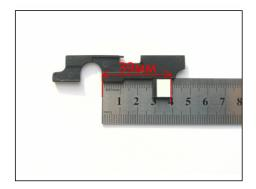
For convenience, first install the "ruler" sticker with the numbers "38 39 40" flush with the cutout on the selector bar and above the tab where the reflective sticker will be glued.
