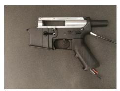
In the program, go to the sensors tab and make sure that all the sensors are working correctly, for this: - manually make a full rotation sector of the gear and make sure that the sensor switching is displayed in the program. When the gearbox is assembled, the operation of the gear position sensor is displayed in color (green and red) on the diagnostic graph;
