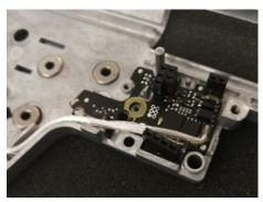
Secure the board with the screw for the contact group. Make sure that the screw does not stick out from the back and will not interfere with the movement of the selector bar.
