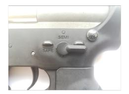
If the AUTO mode is not turned on for you, and the SEMI and SAFE modes work, then you need to move the sticker, reducing the previously set distance of 39mm by 1 mm, i.e. make it 38mm, which corresponds to the green marks on the "ruler" sticker.
