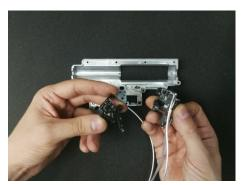
Install the Desire bottom board to which the wires fit. Make sure that it is adjacent to the wall of the gearbox and nothing prevents it. Route thin wires first, then wire from the battery to the board, and wires leading to the motor on top.
