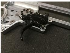
Attach the second wall of the gearbox and make sure they fit tightly without any effort. After that, make sure that the sector gear rotates freely and the trigger is pressed freely, without clinging to the elements on the board.
