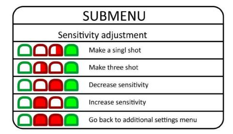
The algorythm sensitibity adjustment is necessary in the following cases:
