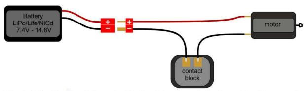
When installing Arm-V pro3, the contact block switches the control voltage only and has no particular load.
